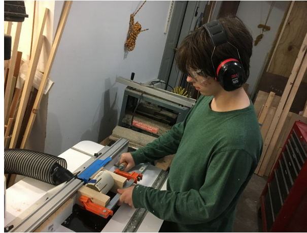
Figure 8. Routing slots in PVC pipe to make gripper section. (Power turned off for photograph.)
