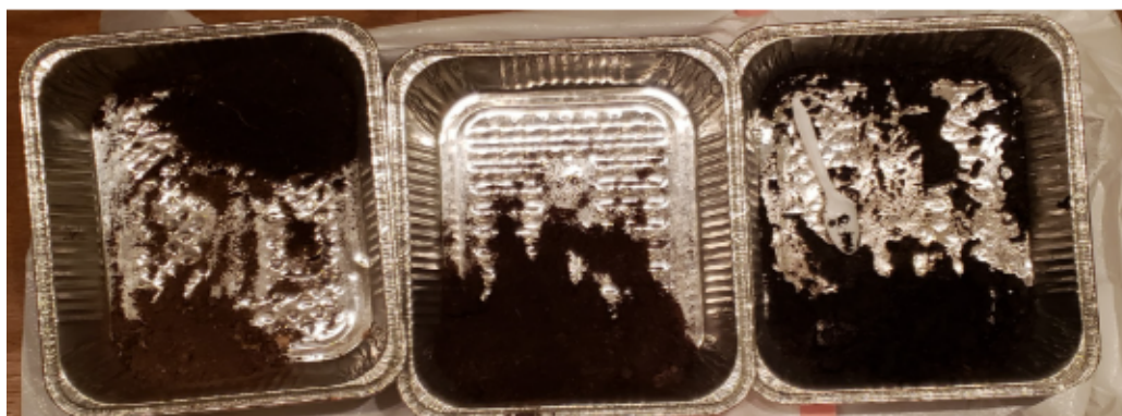
Figure 6. Dry, normal, and wet soil samples used to test the robot.
